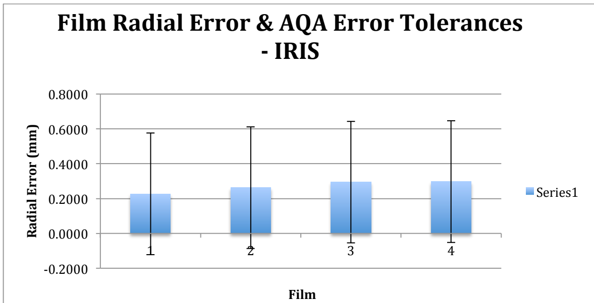
Figure 4.5.1 IRIS Tolerance Stack Up - Maximum & Minimum Radial Error
